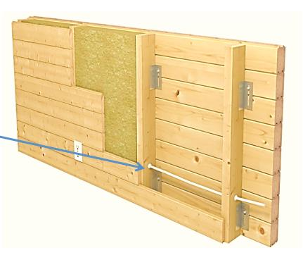
Wiring installed in studs using the same method as regular construction
