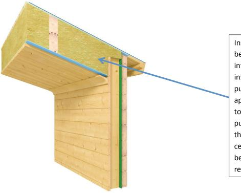
Insulating the ceiling can be done from the interior by placing insulation between the purlins and then applying a cover board to the underside of the purlins. Insulating from the underside reduces ceiling heights. Walls can be increased in height if requested.
